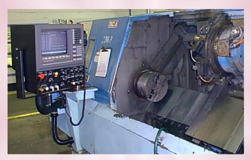
These packages are designed to retrofit Jones & Lamson A, B, C & D size lathe models currently equipped with NC or CNC controls. The packages are completely pre-engineered and field proven, *control only* retrofit; designed to be installed in approximately 40-hours at the your location.
